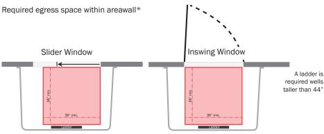
Minimum size areawell for both slider and inswing window are 42" x 36" with a Life-Step  $^{\text{TM}}$  ladder.
